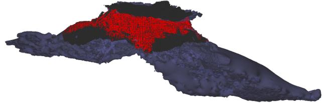
Fig. 3: A partially explored OG from a simulation trial with occupied (red) and free (black) cells and 0.1 m resolution.
